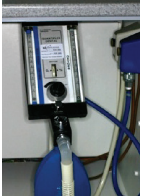
Figure 11 (above). 35-year-old RA Quantiflex (now Matrix) MDM head used in the authors' practice, which is regularly serviced Figure 12 (below left). Turning a glove inside out when touching controls Figure 13 (below). A loose bag over controls
